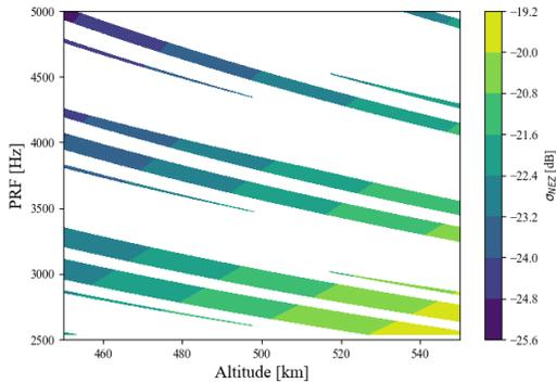
Fig. 2. PRF vs Altitude vs  $\sigma_{NEZ}$  tradespace. The minimum PRF is about 2500 Hz to satisfy to the Nyquist sampling criteria. Altitude uncertainties in mission is expected either due to (1) launch orbit uncertainties (2) gradual decay of altitude during mission lifetime.
