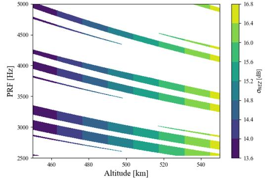
Fig. 3. PRF vs Altitude vs half-power beam illuminated Swath. Swath width increases with increased altitude at the expense of the  $\sigma_{NEZ}$ . But the later can be compensated by operating at higher PRFs or larger transmit pulse widths.
