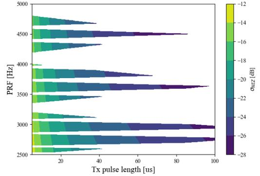
Fig. 4. PRF vs transmit pulse duration vs  $\sigma_{NEZ}$ . This tradespace plot is drawn for a constant desired swath of 10 km. A larger transmit pulse has fewer regions of operable PRF, but with the advantage being that the  $\sigma_{NEZ}$  is improved.
