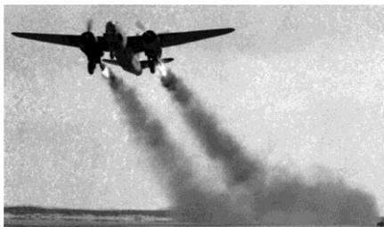
*Douglas A-20A Havoc takes off using liquid-propellant rocket JATO from Muroc (now Edwards AFB) [Courtesy JPL 383-93 1942].*
