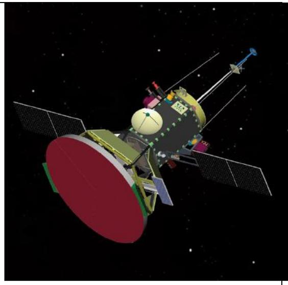
Figure 2. Solar Probe+ shown with primary solar array panel deployed (size: approx. 2.7m diameter heat shield x 3.0m w/o HGA, total weight 481 kg) .
