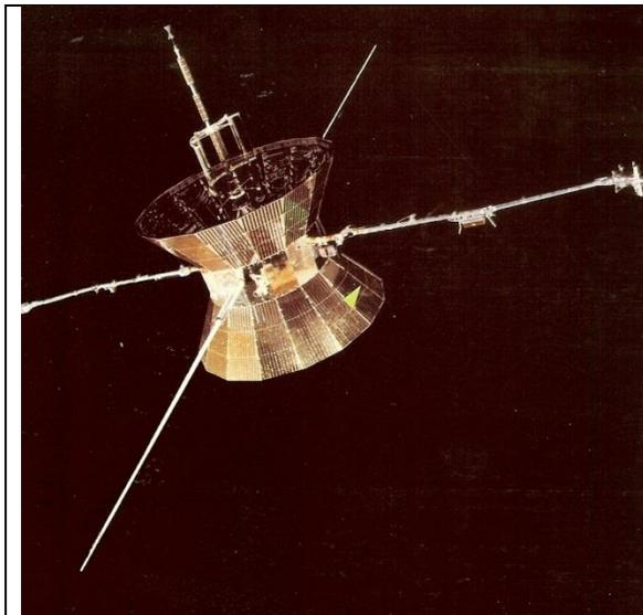
Figure 1. Helios-A in-flight configuration (size: approx. 2.77m cone diameter x 4.21 overall height, total weight 369 kg)
